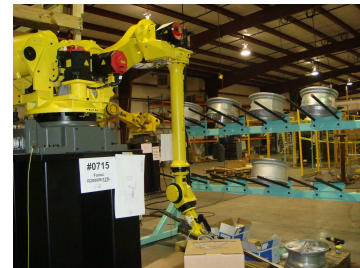
Furnace Load and Queue Rack Fanuc R2000iA
