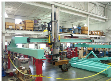
Gantry for Furnace Unload 4 axis Gantry, 800kg Payload
