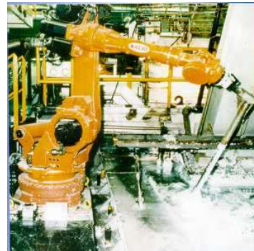
Drossing with NACHI 6-axis robot
