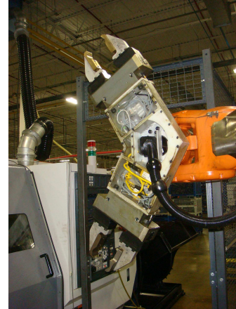
The end-of-arm tool for the heavy cell
