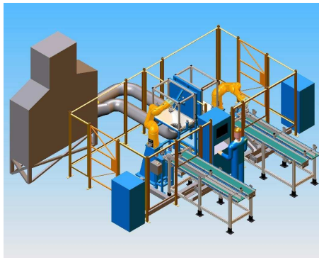
3D Layout Dual Deburring Cell
