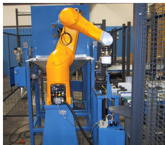
Pump Diffuser Finishing Cell Staubli RX90
